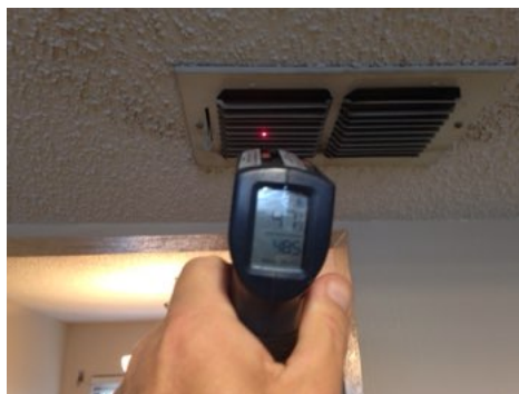
Cooling System - Supply is 46 degrees.
