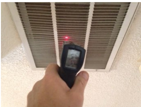
Cooling System - Return is 57 degrees.
