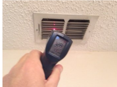
Heating System - supply 128 degrees.
